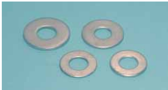
These are all 1/2 inch flat washers. The lower right one is SAE standard. The other three are from different batches of USS standard. Note the wide disparity among the USS washers.
