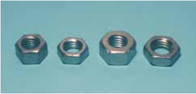
Left to right: nut, jam nut, heavy nut, heavy jam nut. All of these nuts fit the same size bolt.
